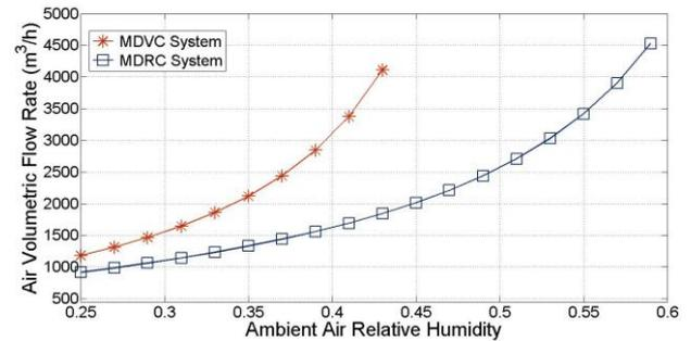
Figure 7: Effect of ambient air relative humidity on required air volumetric flow rate
