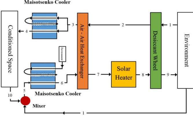
Figure 1: MDVC air conditioning unit configuration
