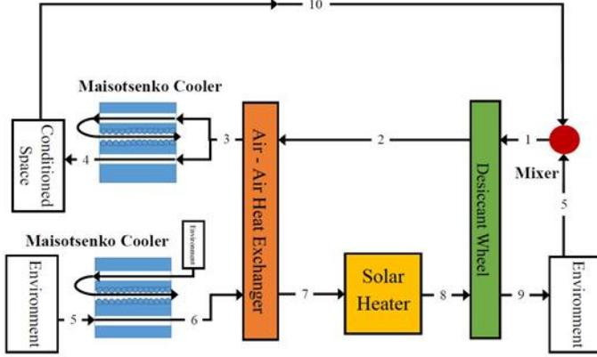
Figure 2: MDRC air conditioning unit configuration
