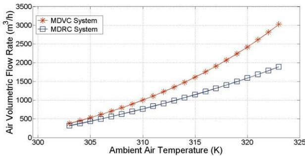
Figure 5: Effect of ambient air temperature on required air volumetric flow rate
