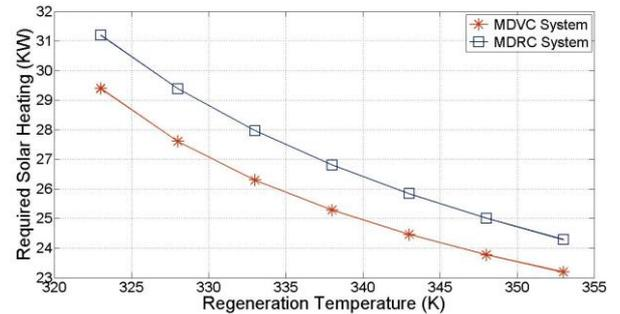
Figure 4: Effect of regeneration temperature on required solar heating
