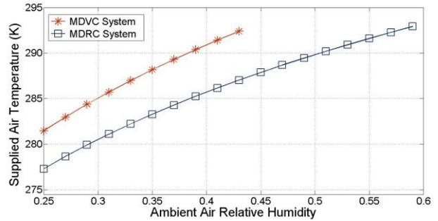
Figure 6: Effect of ambient air relative humidity on conditioned space supplied air temperature
