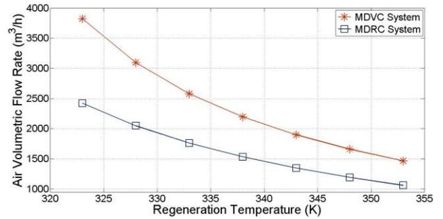
Figure 3: Effect of regeneration temperature on required air volumetric flow rate
