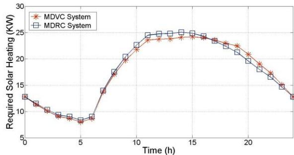
Figure 11: Required solar heating for Abu Dhabi throughout a day
