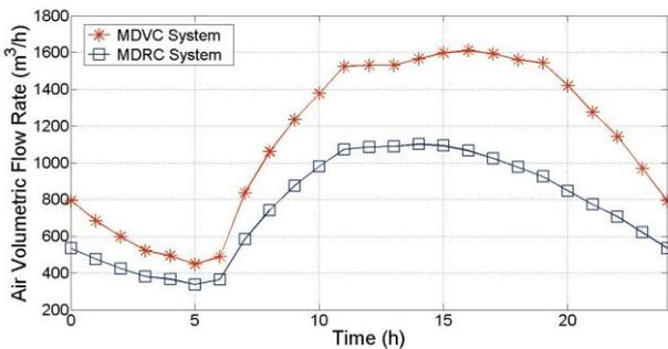
Figure 10: Minimum Required air volumetric flow rate for Abu Dhabi throughout a day
